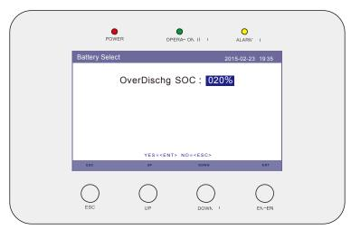
Figure 5.33 Over discharge SOC.
