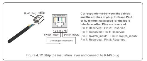
3. Connect RJ45 to DRM (logic interface) .
